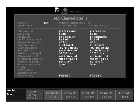
Figure 3-39: Channel Status display in Text format
