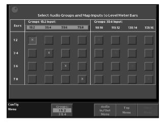
Bar labels when Audio Program Type is set to Stereo Pairs
